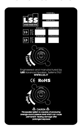
In the connection panel there are two Speakon NL4 connectors referred as 'INPUT' and 'LINKOUT'.
