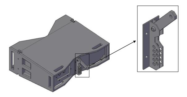
Plates of two overlapping speakers must be connected via the connecting bracket. Align the holes in the desired position, then secure them with the quick release pins.
