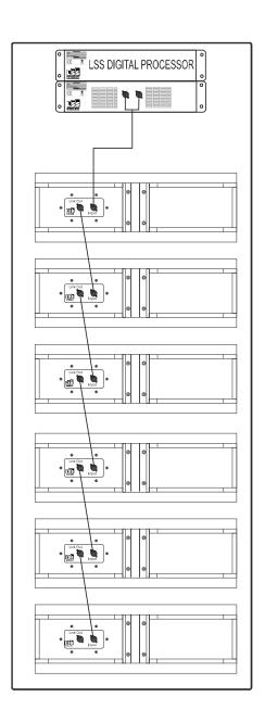
HDA24 system operating mode is only Bi-Amp (LF 1- 1+; HF 2- 2+) and needs an external digital processor with custom setup provided by LSS. If your amplifier can manage a 2 Ohms Load and has sufficient power, it is possible to connect a maximum of 6 speaker in parallel (total impedance will be 2 Ohms).
