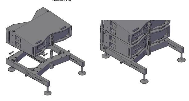
In case of installation in Flying mode, use the bumper without extensible bars and feet, attach the speaker to the sides via connecting bracket, then connect the rear bracket adjusting the inclination.
